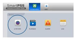
2) Before viewing cameras select the view you wish to use. You may select the single image view to display one camera at one time or select other image views to display up to 64 cameras on the screen at one time.
